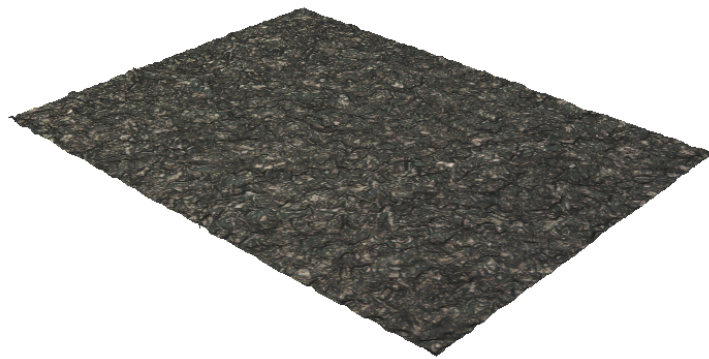
Figure 3.3 – 3D image of inside PM surface generated by the Alicona IF Portable.
