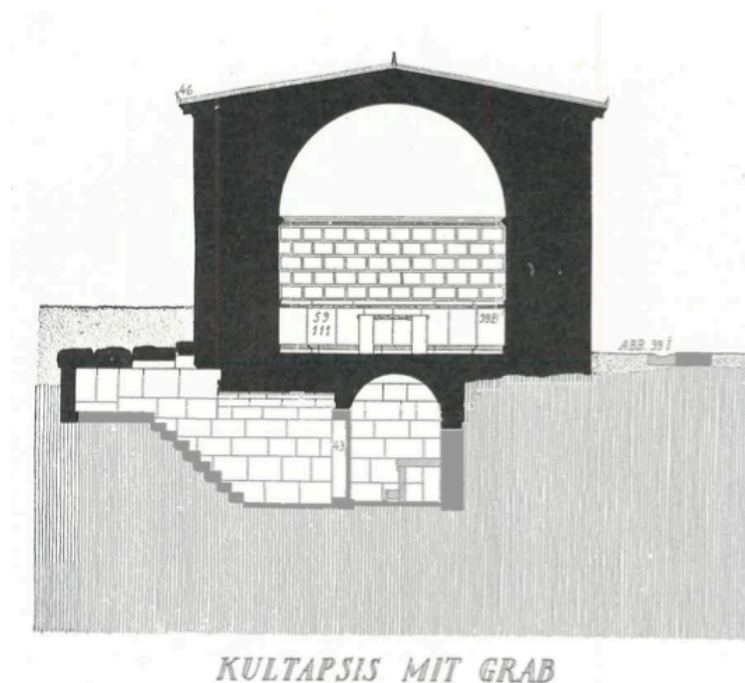
Figure 37: Reconstruction of “Kultraum” and tomb with vaulted ceilings (Dyggve et al. 1934).
