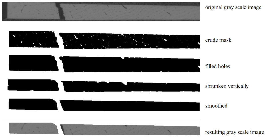
Figure 21: Binary mask (white) used for background removal. The crude mask is composed of the four clusters corresponding to the lowest pixel intensities after K-means clustering of the original gray scale image using six clusters.
