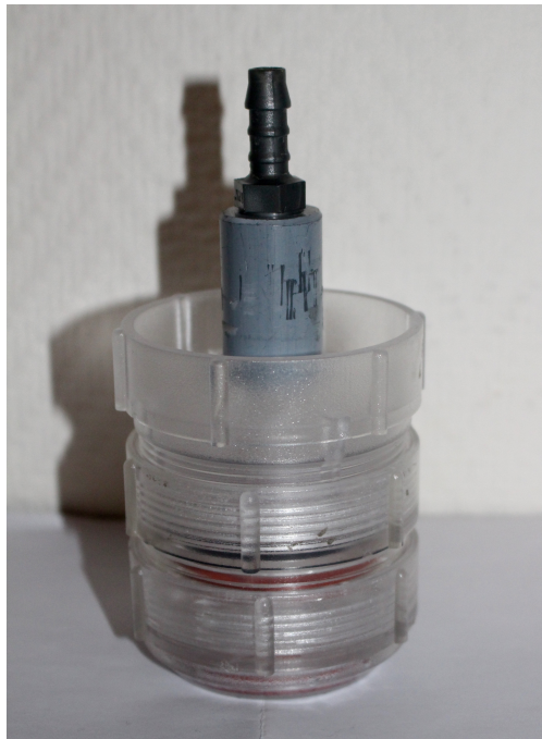
Figure 11: An image of a stacked filter unit (SFU).
