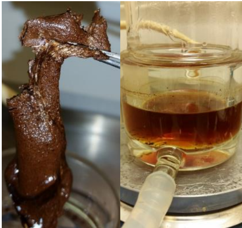
Figure 4.14. The heavy phase can be picked up with a pair of tweezers and is slowly dragged out by its own weight. The light phase is very clear after the heavy phase have been removed.
