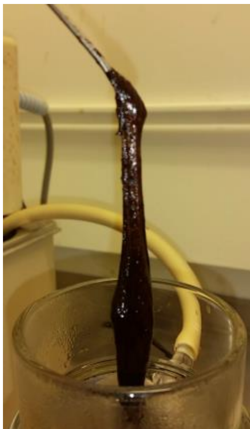
Figure 4.16. One experiment with acidulation powder was successful and yielded a liquid heavy phase.
