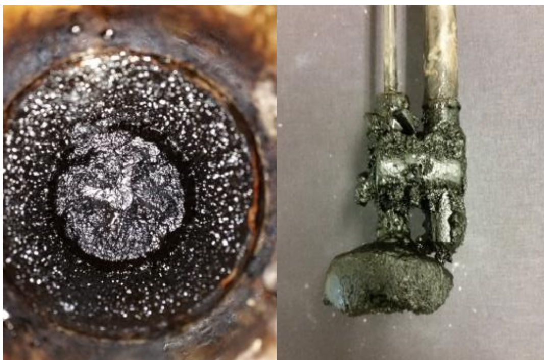
Figure 4.7. 5 bar differential pressure did not yield a heavy liquid-phase for any temperature. This can be seen as the precipitate in the reactor bottom are not smooth and the stirrer has no solidified droplets. Photos are of 130/5.
