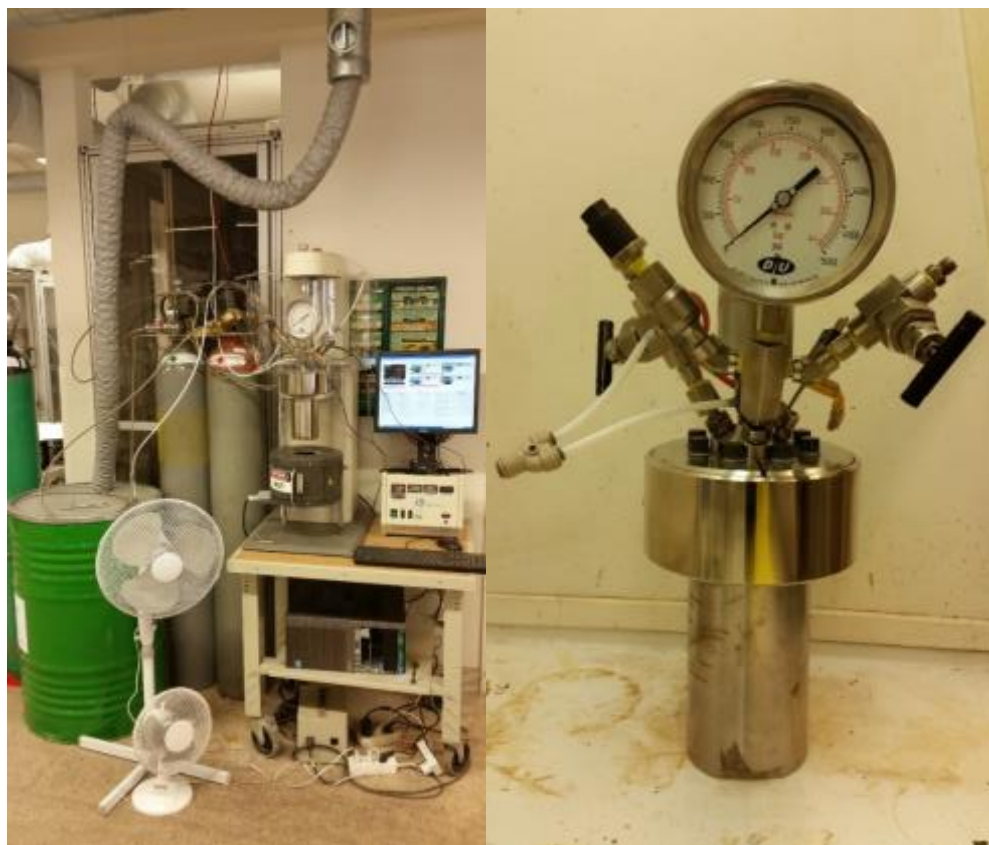
Figure 3.1. On the right is the Parr reactor used during trials and to the left is the entire setup as it was during an experiment.
