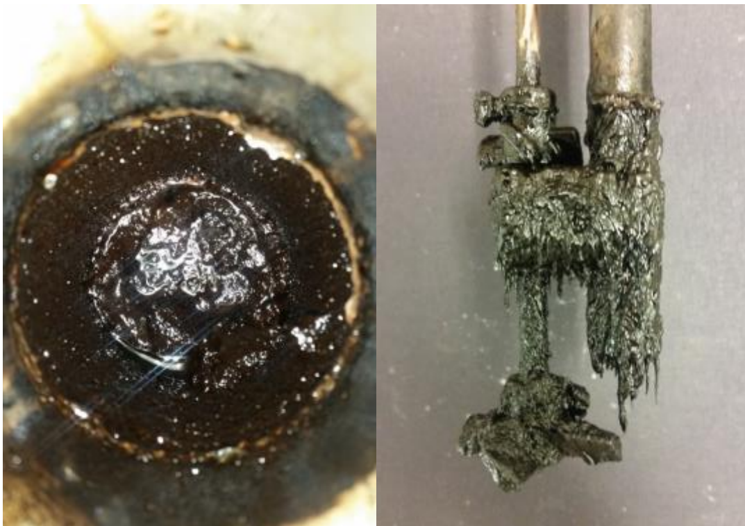
Figure 4.6. 110/15 was stored in the fridge overnight and the top of the solidified heavy liquid-phase had been dissolved by the light liquid-phase.
