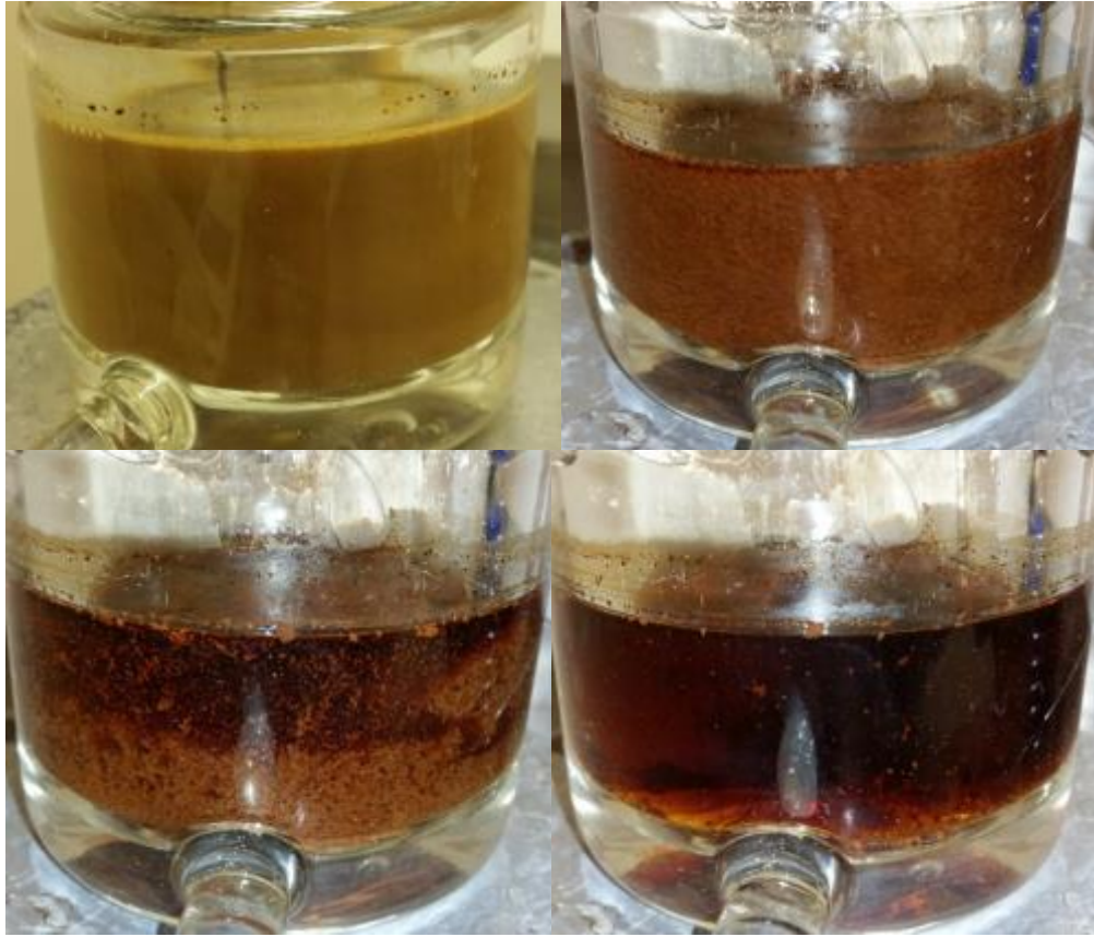
Figure 4.13. Experiments using LignoBoost powder successfully separated into two phases.
