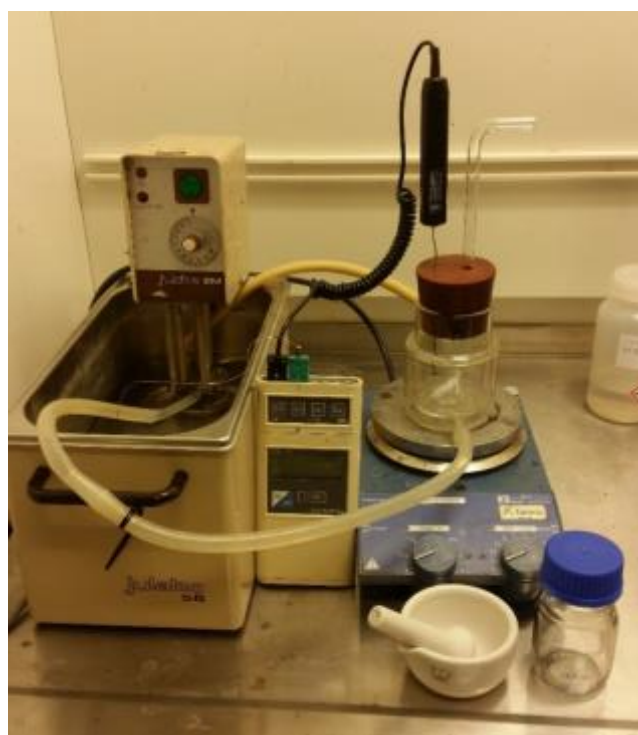
Figure 3.2. Equipment setup used for the ALPHA purification trials. A heated water bath pumps hot water through a mantled beaker that is placed on a stir plate.
