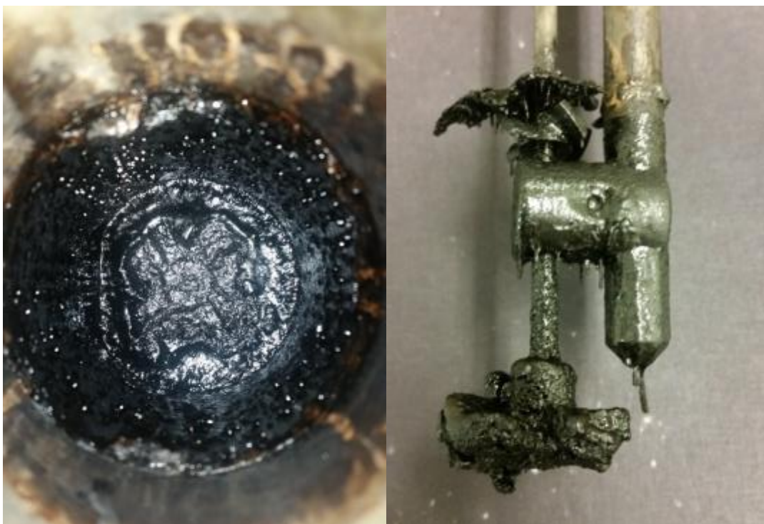
Figure 4.8. 150/15 shows the least amount of solids on the stirrer. The top stirrer has a "hat" with small droplets hanging underneath.
