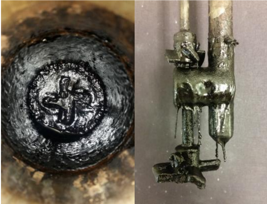
Figure 4.5. 130/15 shows clear evidence of the heavy liquid-phase. A smooth surface in the reactor bottom and solidified droplets hanging from the stirrer.
