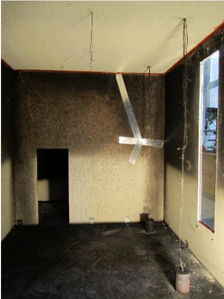
Figure 26: Thermocouples inside the test room.
