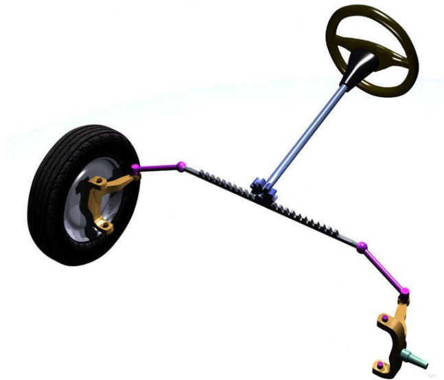
Figure 3: Illustration of a rack and pinion setup [22].
