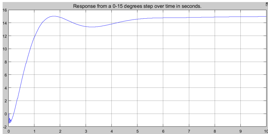
Figure 19: Step response, 0-15°, for the controller with parameters operating from 1.1 to 11 km/h. This was done using MATLAB.
