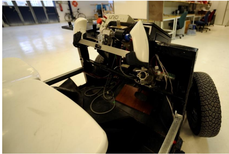
Figure 2: The joystick setup of the test vehicle.
