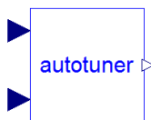
Figure 3.1: The auto-tuner block with two inputs and one output. The inputs to the block are the process output, y , and the set point y_s . The output is the output signal generated by the auto-tuner, u .
