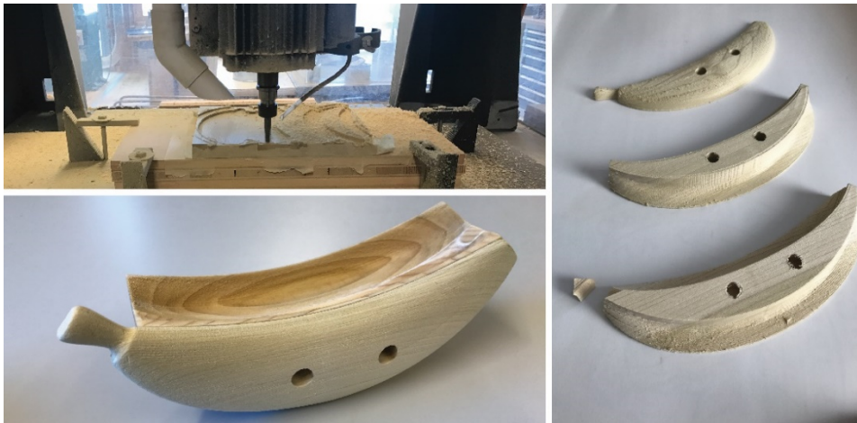
Figure 8.13 CNC-milling of bananas in three pieces.
