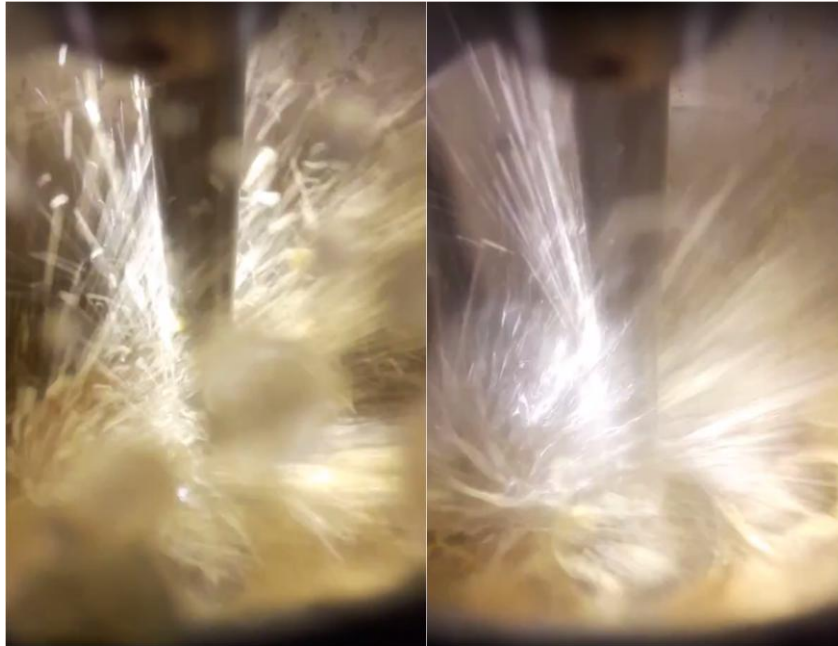
Figure 4.17: Splashing when the oil enters the mixer, a second before the oil covers the window. Left: Oil inlet flow rate of 3.6 kg/s and tip speed 8.3 m/s. This experiment resulted in proper mayonnaise. Right: Oil inlet flow rate of 4.4 kg/s and tip speed 8.3 m/s. This resulted in broken mayonnaise.
