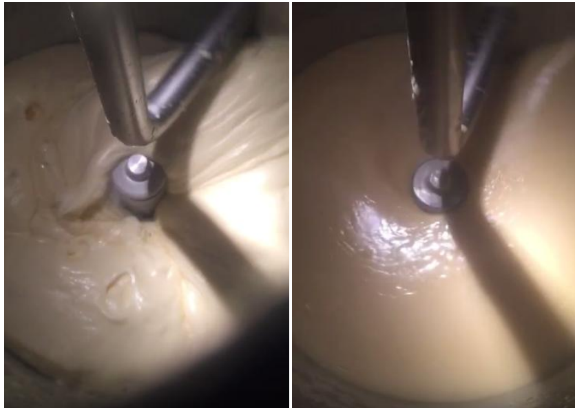
Figure 4.15: Mayonnaise after the coarse emulsion step. Left: Standard mayonnaise made with the coarse emulsion tip speed of 8.3 m/s. Right: Mayonnaise made with the coarse emulsion tip speed of 1.4 m/s.
