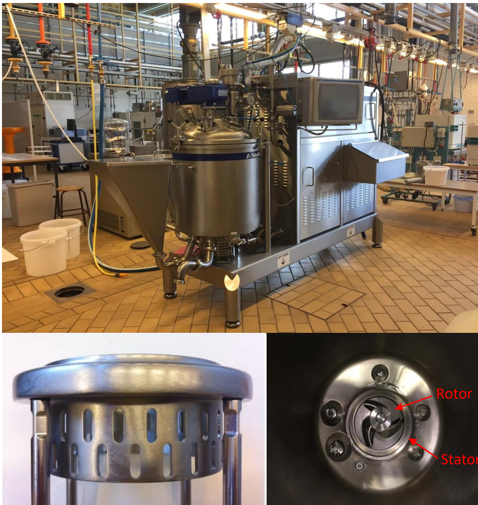
Figure 3.1: Above: the mixer from the side. Left: stator with 5x14 mm slots (Andersson, 2015). Right: inside the vessel of the mixer with the rotor and stator marked.
