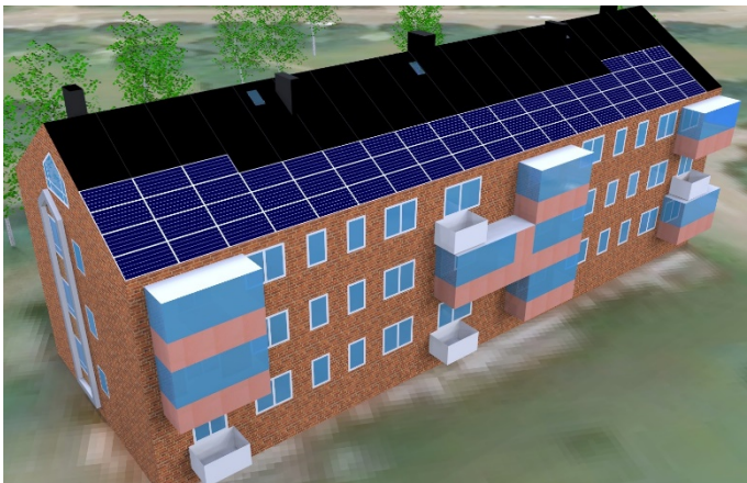
Figure 4.18: Visualization of the best case system design in case of Edwin Berlings gata 2.
