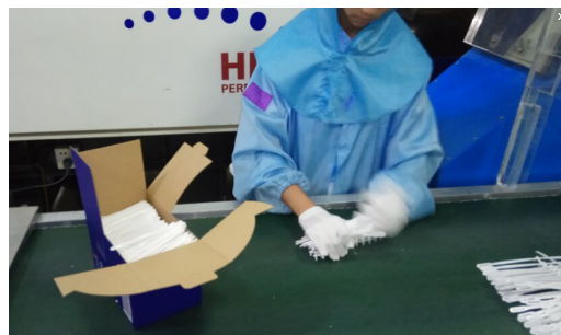
Figure 22. Stirrers were packed manually inside primary cardboard box
