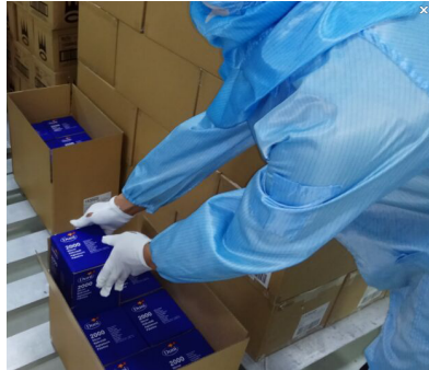
Figure 23. Primary boxes were manually filled inside the corrugated box
