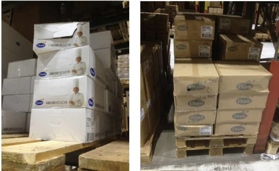
Figure 1. Damaged secondary packaging in Duni due to strength reduction issue
