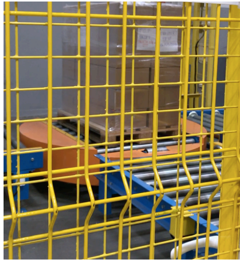
Figure 37. Two conveyor connected, from rotating orange conveyor to roller conveyor
