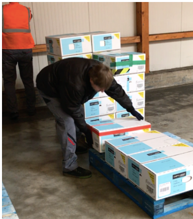
Figure 42. Boxes were manually transferred between different types of pallet
