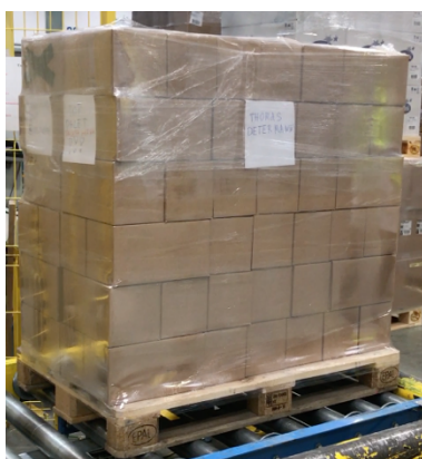
Figure 16. The condition of tertiary packaging after gone trough plastic wrapping process
