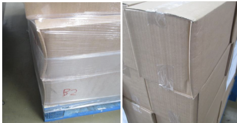
Figure 33. Picture taken at Smithers Pira, dented vertical edge observed at product A.
