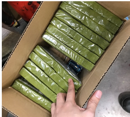
Figure 4. Installation of data logger inside the package
