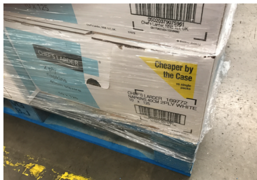
Figure 49. Self-open perforation observed happened at shelf ready packaging of product B
