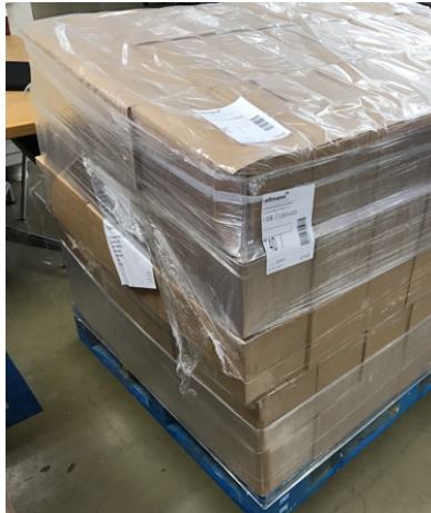
Figure 35. Tear off plastic wrap observed in Smithers Pira
