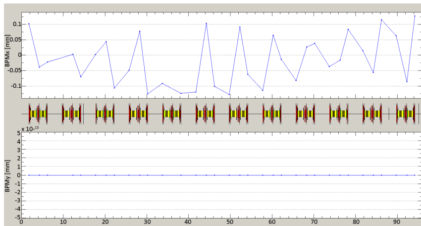
(b) Orbit response of the simulation when applying a horizontal kick to the beam. The first horizontal corrector was used, with a kick corresponding to 1 A.
