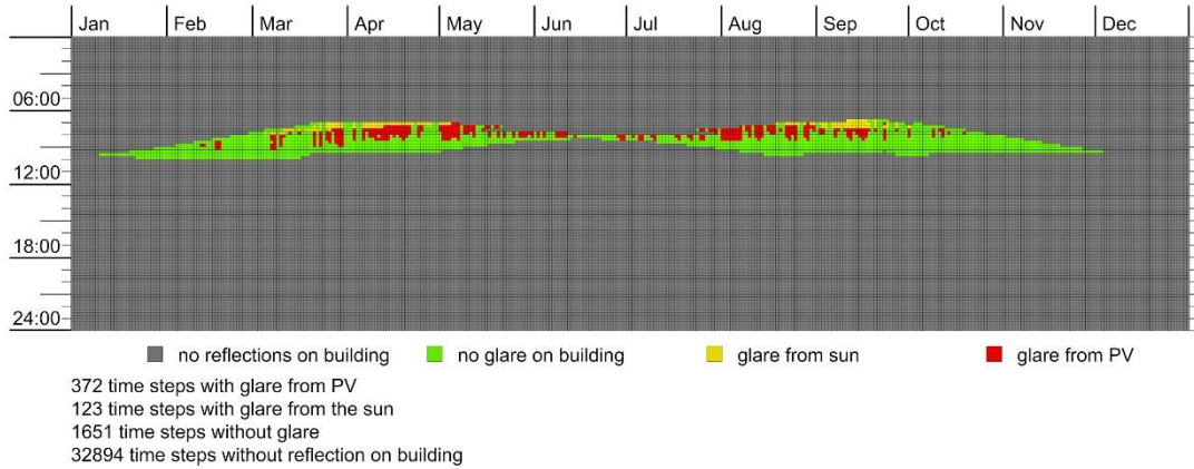
Figure 4.4: Temporal map of the study results for the area 6 of the building surface (area 6 is shown in the visualization on the right in Figure 4.3)
