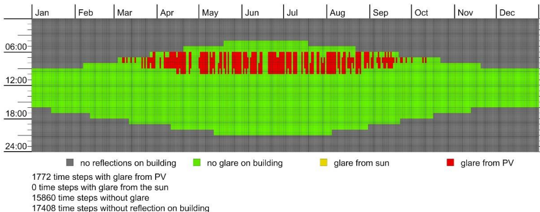
Figure 3.7: Temporal map showing the results of the DGP study, all glare is marked as glare from PV
