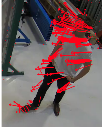
FIGURE 3.7: Example of the extracted optical flow. The arrows represents the pixel velocity amplified by 10.
