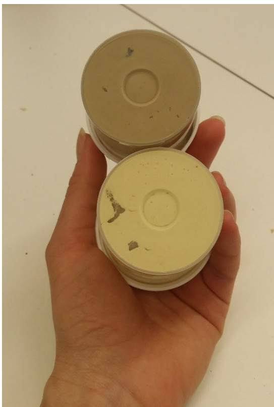
Figure 19. The products of the two UF-trials with and without \text{Na}_2\text{S}_2\text{O}_5 . Above: UF product w/o \text{Na}_2\text{S}_2\text{O}_5 , below: UF product with added \text{Na}_2\text{S}_2\text{O}_5 .
