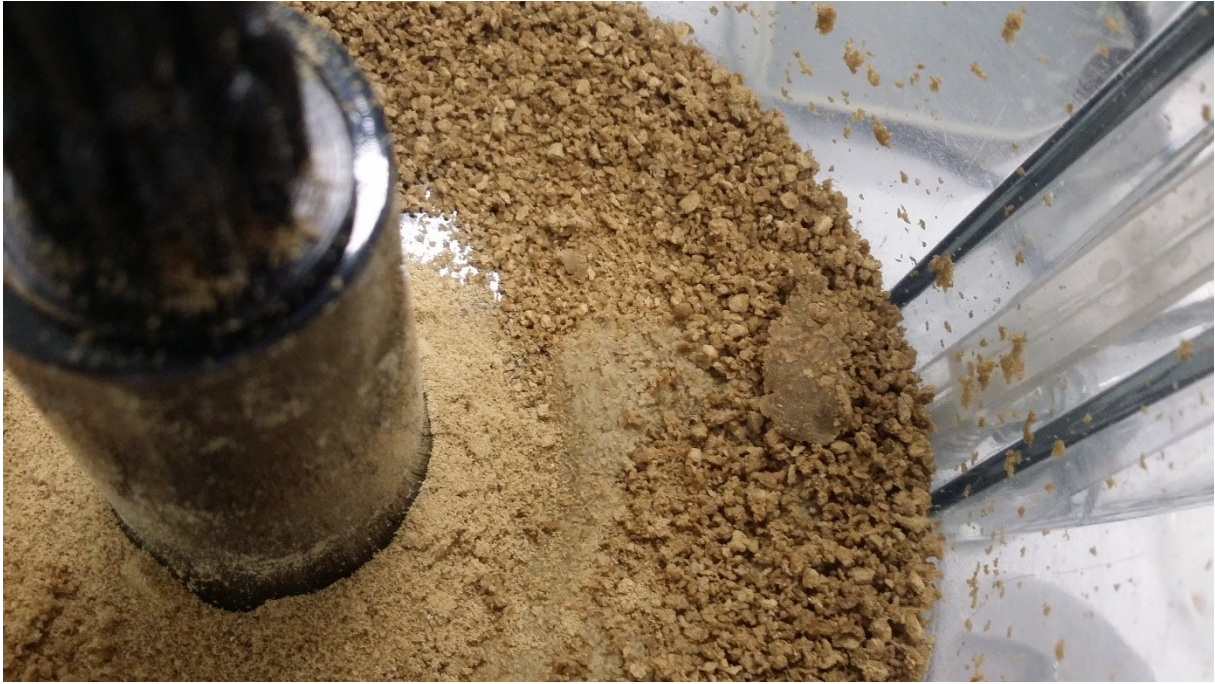
Figure A1. The dough used in the extruder. This is right after it had been mixed with water in the mixer. The FD RSP mixed with 50% water.
