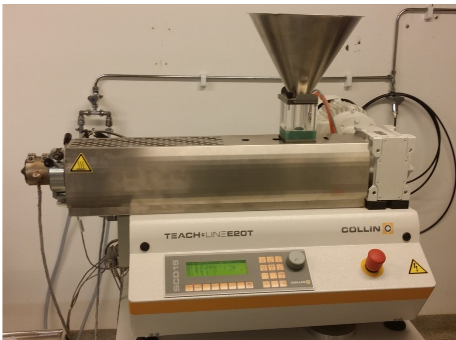
Figure 7. The single-screw extruder used in the current thesis.
