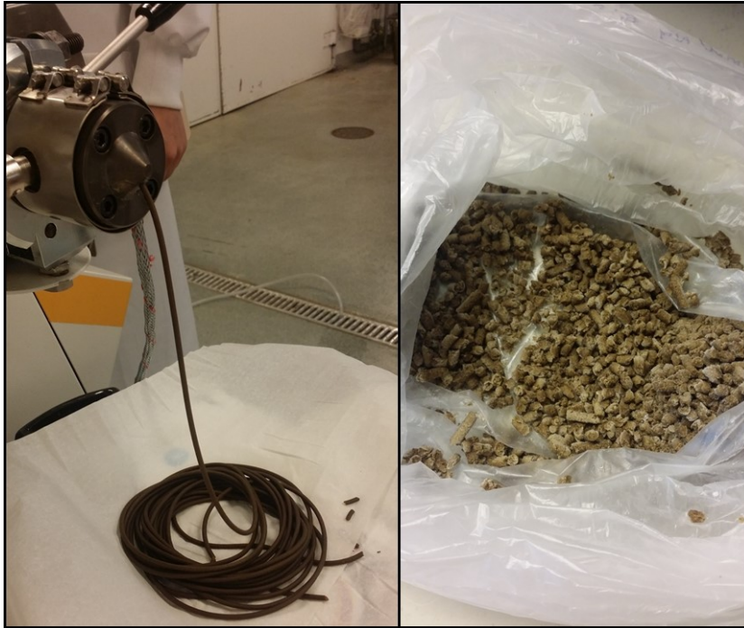
Figure 28. Left: The extruded product with the round die and 100°C with a screw speed of 40 rpm. Right: The extruded product with the round die and 120°C with a screw speed of 45 rpm.
