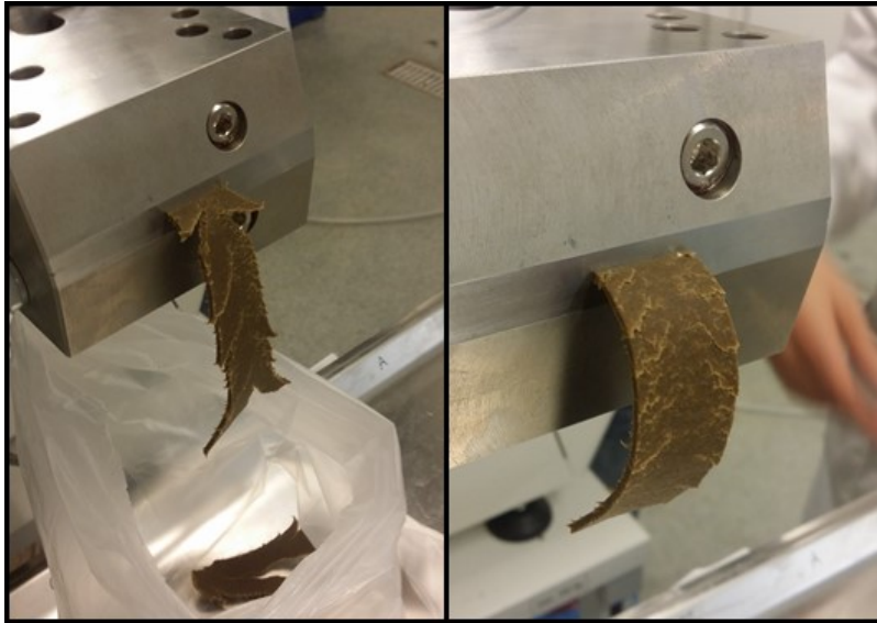
Figure 29. Extruded products with cooled flat die. Left: At 100°C and screw speed 70 RPM. Right: 120°C and screw speed of 70RPM.
