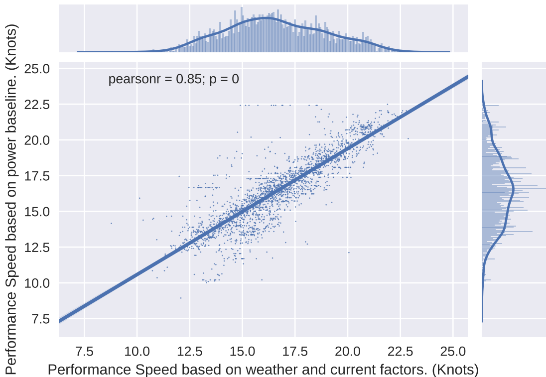
Figure 3.6: The correlation between the true speed calculated using main engine power and performance speed calculated using weather and current factor are heavily linearly correlated with a PCC of 0.85.
