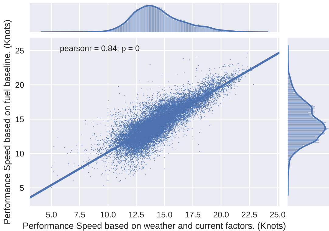
Figure 3.2: Plotting the performance speed calculated using weather and current factor along with the fuel based baseline speed. They are heavily correlated with a PCC of 0.84.
