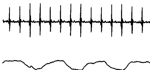
Figure 10 – The first signal is an ECG signal with a clear QRS amplitude variation that resemble the respiration (second signal) [2].
