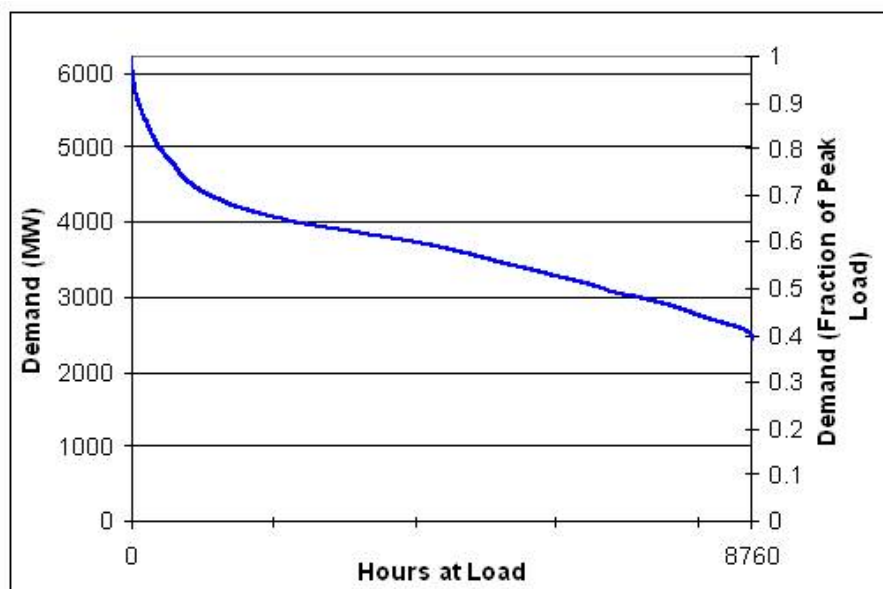
Figure 3 - An example of a typical load duration curve of one year, on which grid dimensioning is normally based on (Mcensustainableenergym, 2011).
