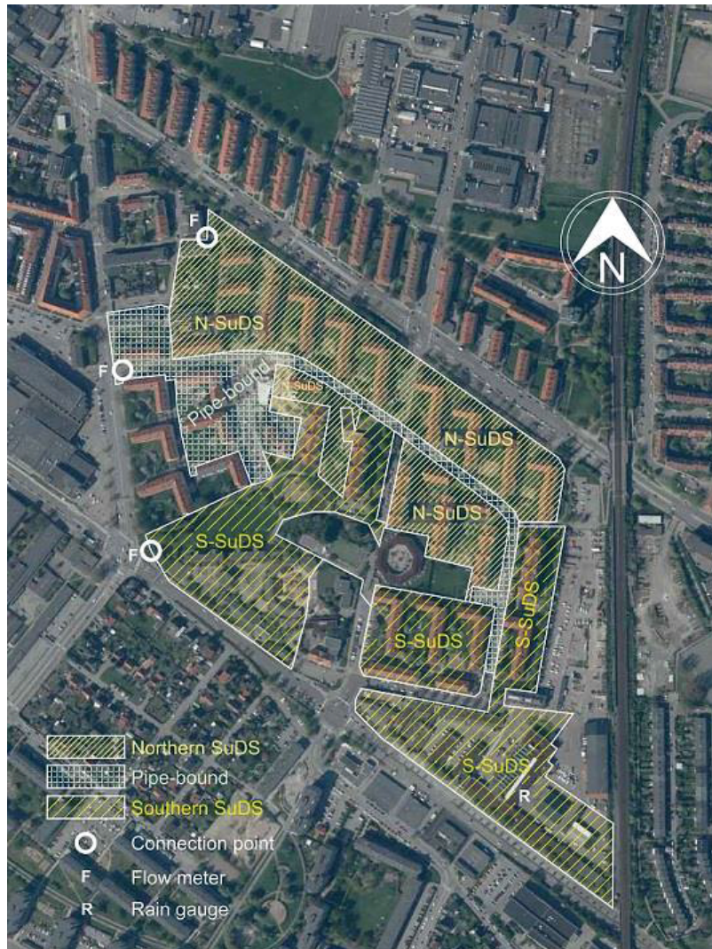
Figure 5.3 Map of Augustenborg marking regions with different drainage systems. Source: Published with kind permission from Salar Haghghatafshar (Haghghatafshar et al., n.d.).
