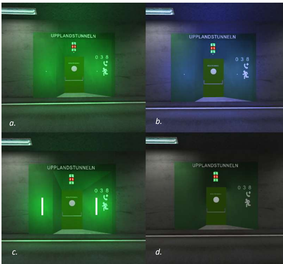
Figure 8. VR emergency exit portal designs. a. Reference scenario (Fast flashing and Single Strobe designs look the same but present variances in the flashing rate and period correspondingly), b. Blue lights, c. 2 bars and d. No lights.
