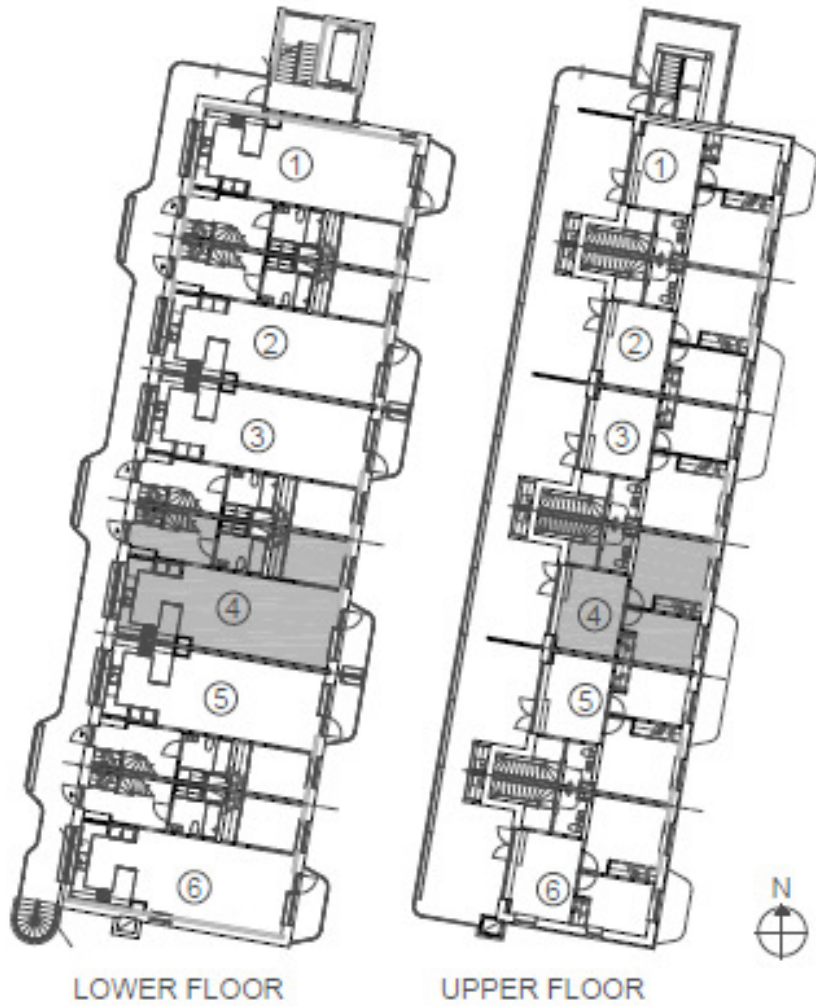
Figure 7- Floor plans of the upper six maisonette apartments of Låghuset. The highlighted apartment is presented more detailed in figure 8.
