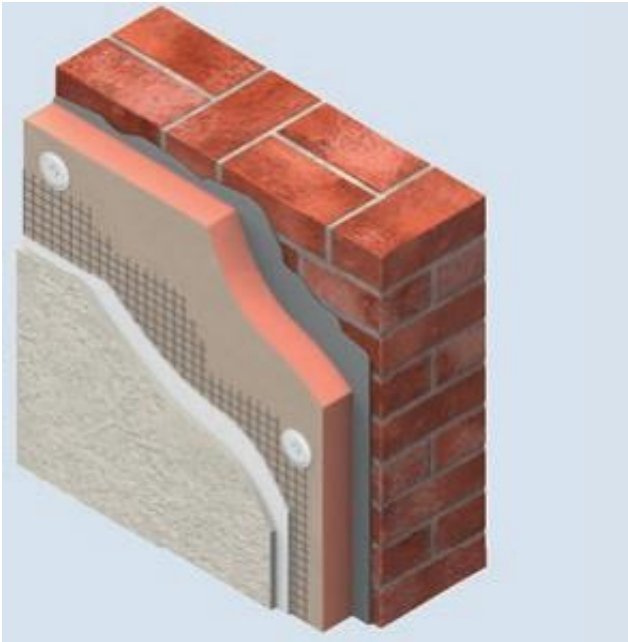
Figure 5.10. Illustration of the different layers included in the renovation measure of the external walls. (Kingspan, 2016)
