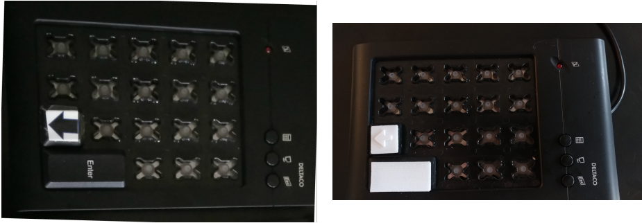
Figure 4.6: L; First prototype of the physical remote. R; Final version with 3D-printed tactile keys.
