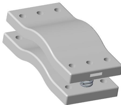
Figure 6.22 The double bracket with push springs for the one-bracket version of Iteration IV .
