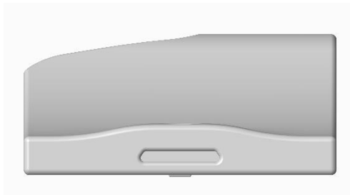
Figure 10.23 The bracket from Iteration VIII shown from the side showing the reinforcement over the hole that also give a hint of where to place the fingers.
