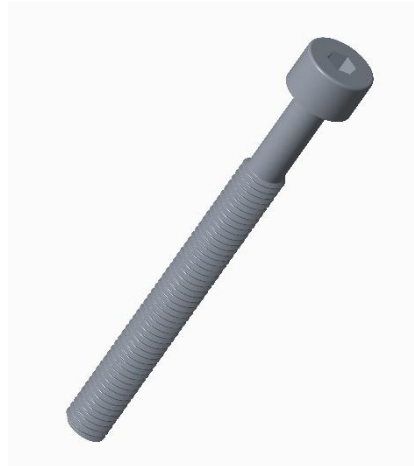
Figure 10.28 The special made anti loss M8 screw.
