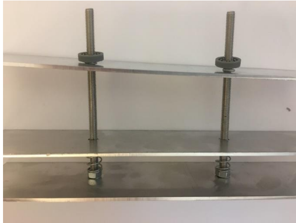
Figure 6.5 An early prototype of the concept of Iteration IV including the snap mechanism and a double bracket with push springs.
