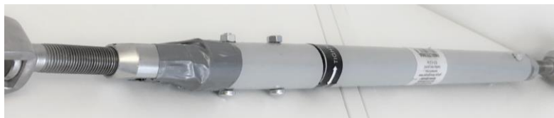
Figure 5.7 The second prototype of detail concept D: Telescope and turnbuckle in the collapsed mode.
