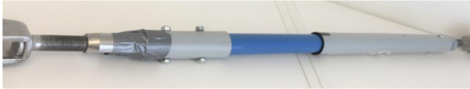
Figure 5.8 The second prototype of detail concept D: Telescope and turnbuckle in the extended mode.
