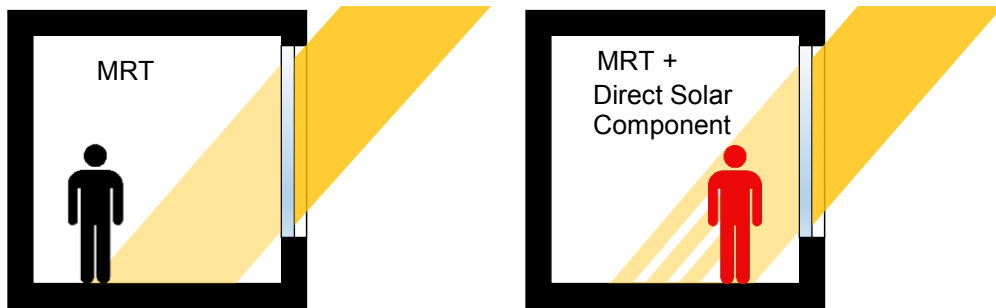
Figure 2. Effect of the direct solar component on the thermal sensation of the occupant
