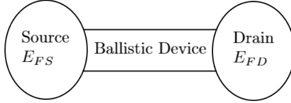
Figure 2.1: Sketch of a ballistic device with source and drain contacts which act as thermal equilibrium electron reservoirs.
