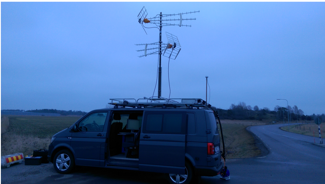
Figure 3.8: Mounted antennas during a live measurement.
