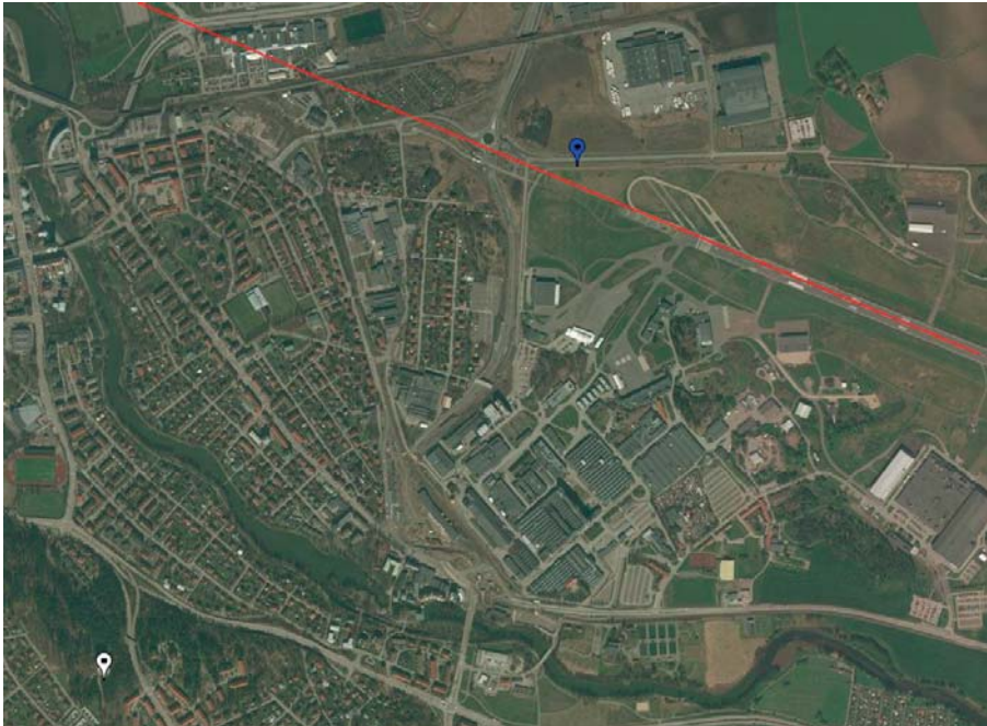
Figure 7.1: Geometry during the measurement at Linköping airport. The white marker is the location of the transmitter, the blue marker is the location of the receiving antenna and the red line is the approximate flightpath of the aircraft.
