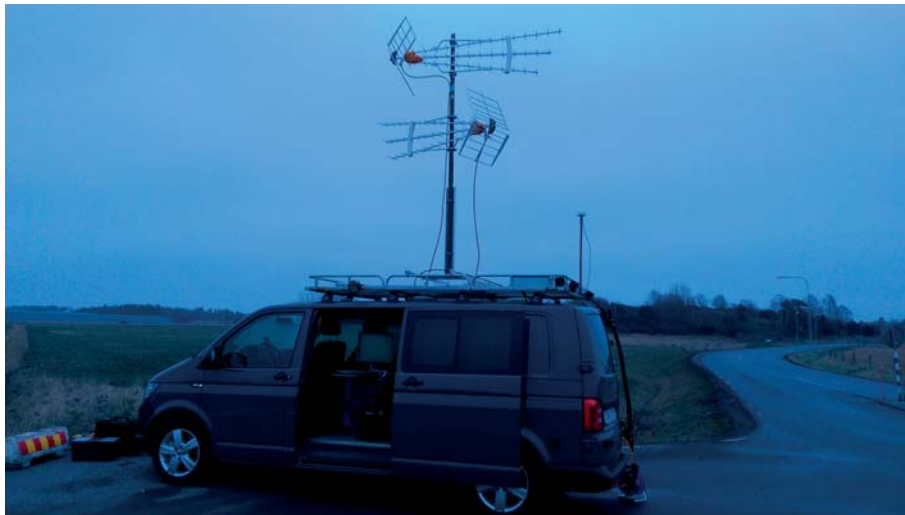
Figure 3.8: Mounted antennas during a live measurement.
