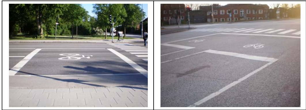
Figure 7: The types of bicycle box
