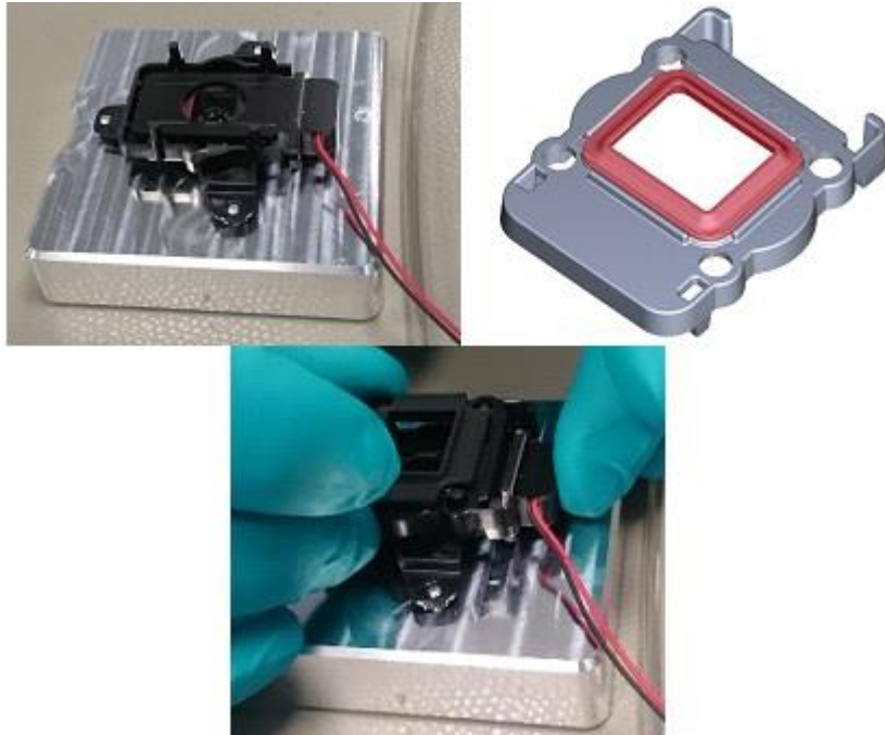
Figure 3.3. TOP LEFT – D-N FILTER is placed in the LENS HOLDER. TOP RIGHT – D-N FILTER LID with SENSOR GASKET. BOTTOM – D-N FILTER LID is snapped in to place over the D-N FILTER.
