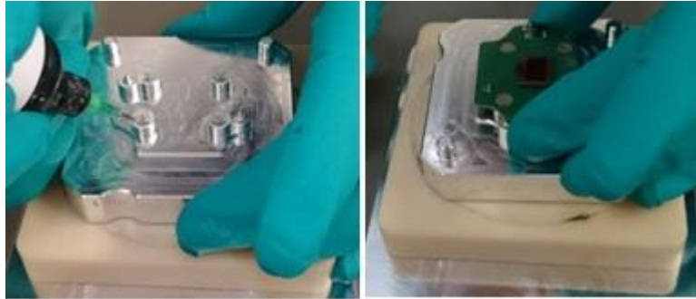
Figure 3.2. LEFT - Adhesive is applied to the ADHESIVE INSERTS. RIGHT - PCB A is placed on top of the inserts in the fixture.
