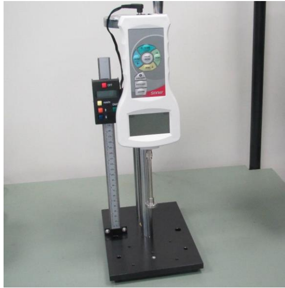
Figure 3.8. The push out equipment. The metal arm pushes down on marked spots on the fixture which transfers the force on to the desired location on the unit.
