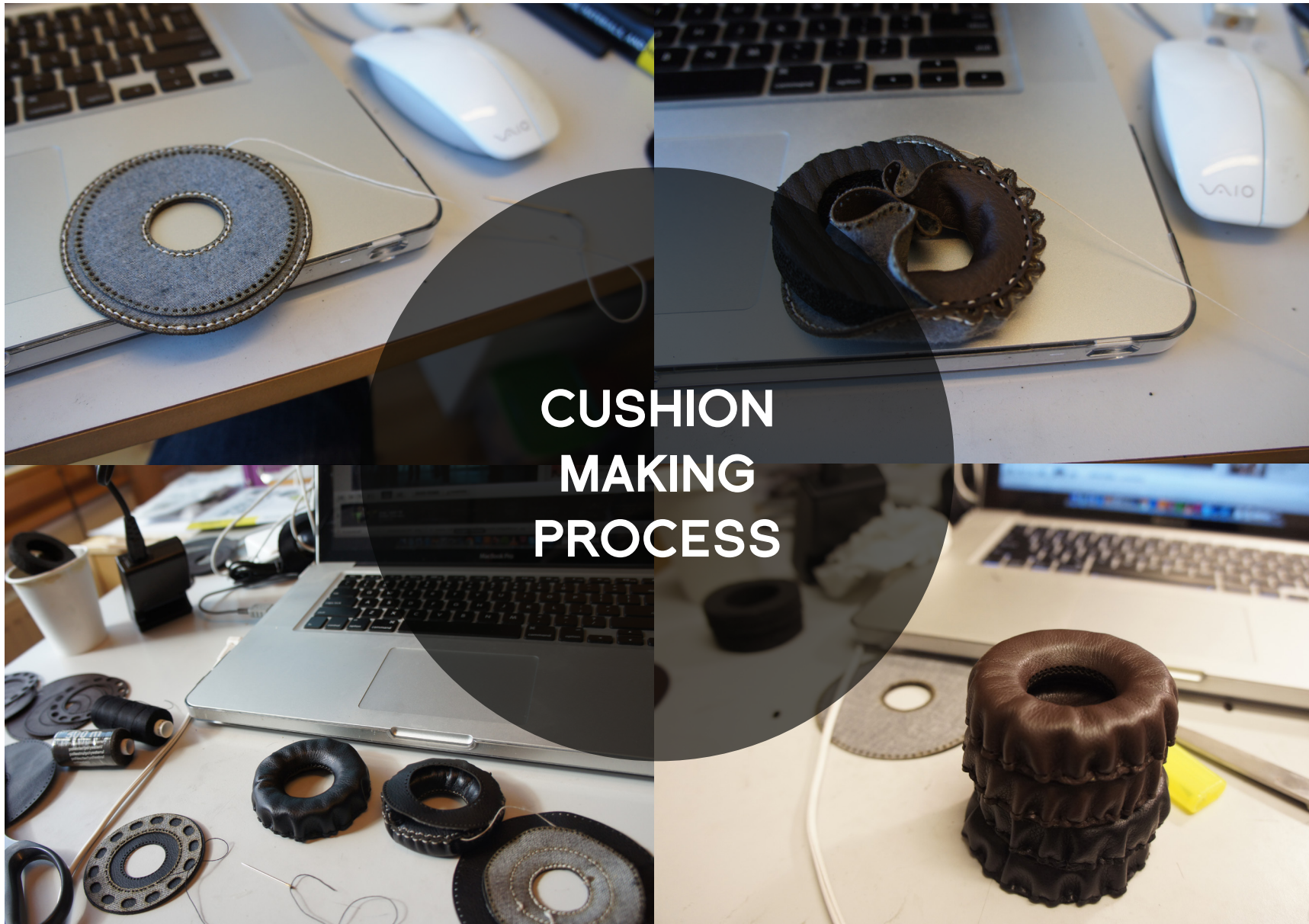
The layouts of cushions has been cut with laser cutter and later sewn by hand.
