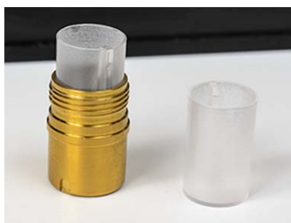
Figure 13. The microcalorimetry stainless steel vial and the sample cup.
