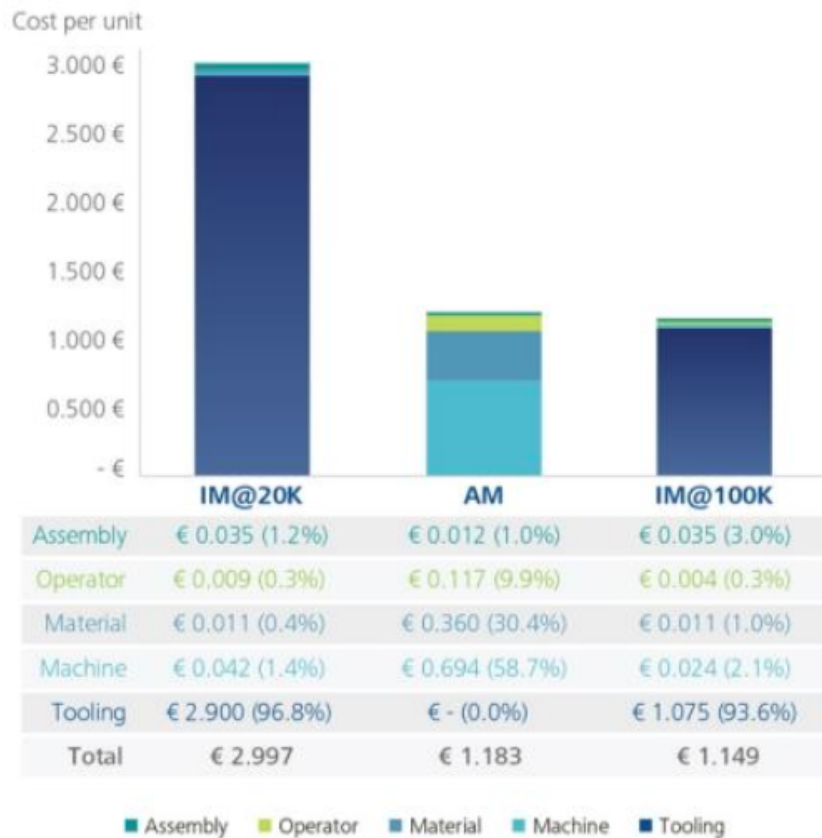
Figure 3.20 Injection molding vs AM [20]
