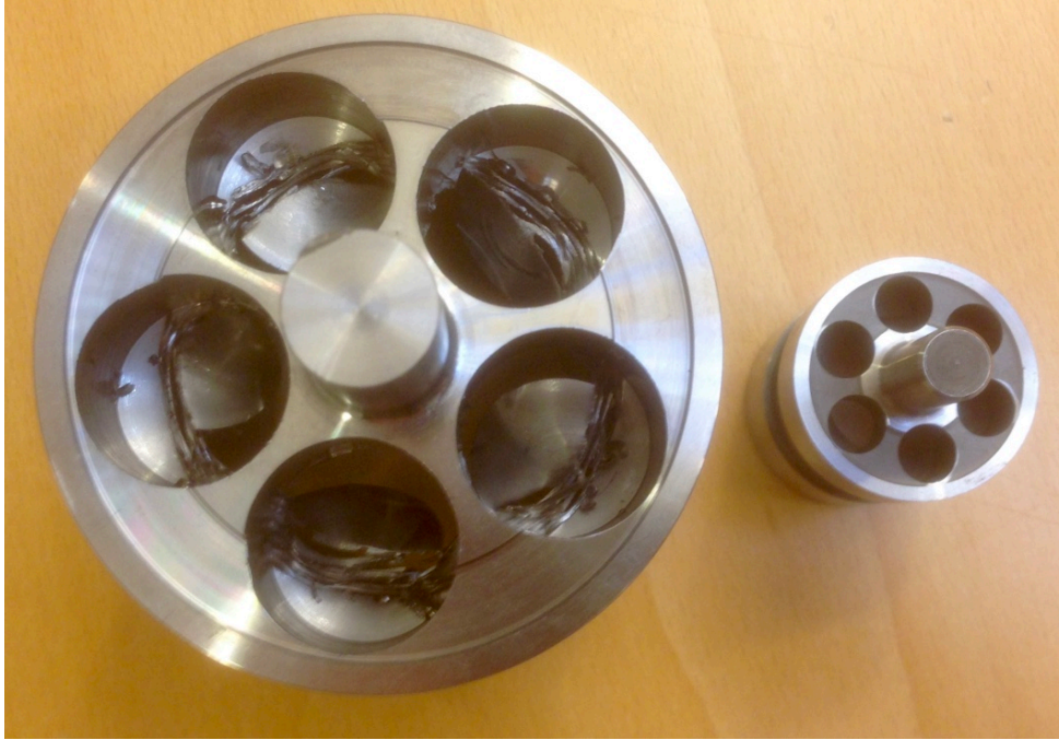
Figure 7.6 Machined component with defects that have arisen in production when deburring the holes.
