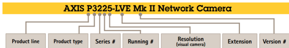
Figure 3.1 Naming structure of the network cameras at Axis [4].
