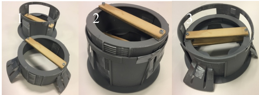
Figure 7.6 The 3D-printed prototype. 1) The two parts individually. 2) The position when inserting the RM through the hole in the ceiling. 3) The position after pressing the handle which enables the wings to flap out and hold the RM above the ceiling.
