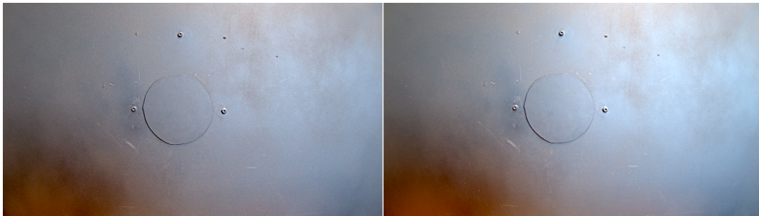
FIGURE 4.9: Picture of the camera image without the cleaning process running (left) and with the cleaning process running (right)
