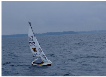
Figure 5.2 ASV Roboat, developed by Austrian Society for Innovative Computer Sciences which uses the Velocity Polar Diagram for planning its path
