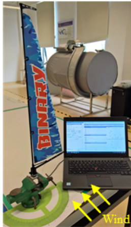
Figure 6.1 The experimental setup of extracting the forces generated by the wind.
