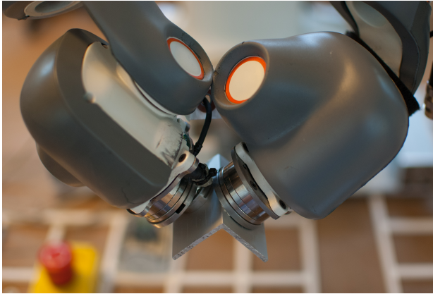
Figure 3.5 The dual arm clamping device with toolchangers on a 90 degree bracket.
