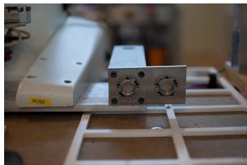
Figure 2: Fixed docking points.
