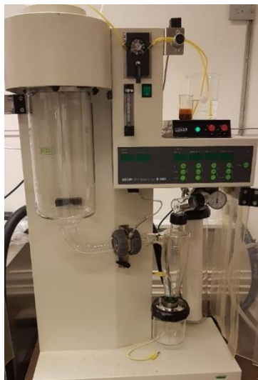
Figure 1.2: The setup of a spray drier
