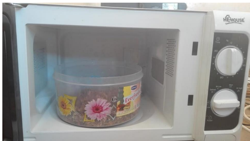
Figure 7: the experimental setup for measuring the moisture content in a microwave.
