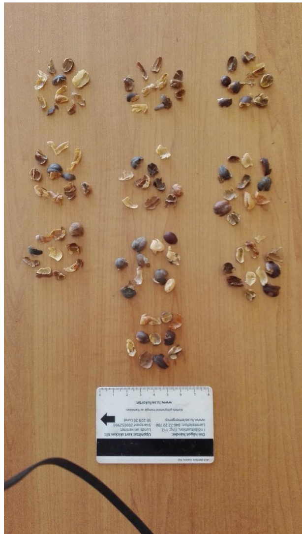
Figure 5: the experimental setup for measuring the particle size and the husks measured.
