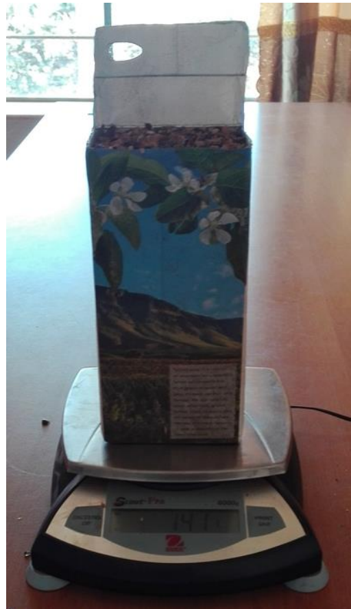
Figure 6: The setup for measuring the bulk density.
