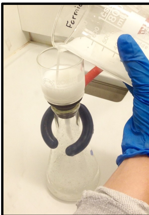
Figure 19. Shows how the biopolymer powder was separated from the acid solution with the help of vacuum filtration.
