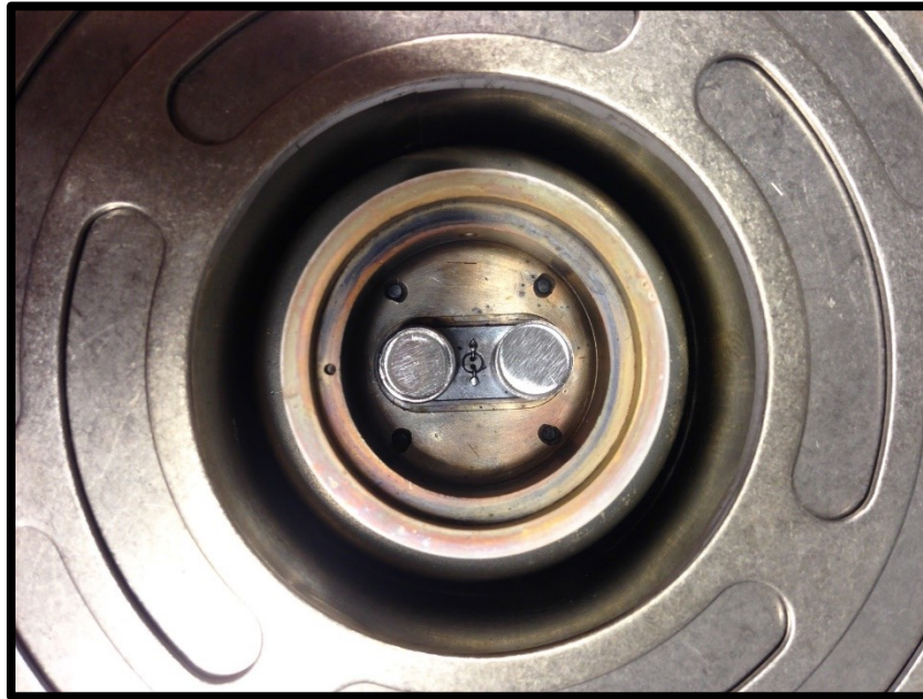
Figure 26. The sample (on the left) and the reference (on the right) placed in the DSC.
