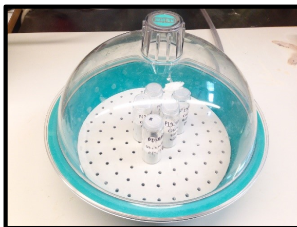
Figure 21. Desiccator with vacuum. Was used when the vacuum oven broke down. Since the temperature was room temperature, the samples were placed there for 48 hours.
