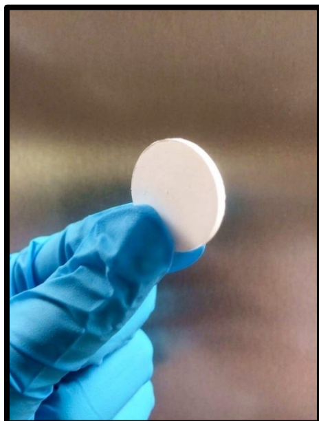
Figure 23. Powder tablet before prepared in the cold press.
