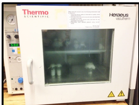
Figure 20. A vacuum oven where the filtered samples were placed at 50 °C for 24 hours to dry before any measurement could be made.
