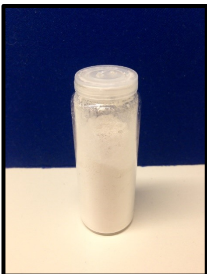
Figure 27. Powder sample after it has been acid treated, filtered and dried.
