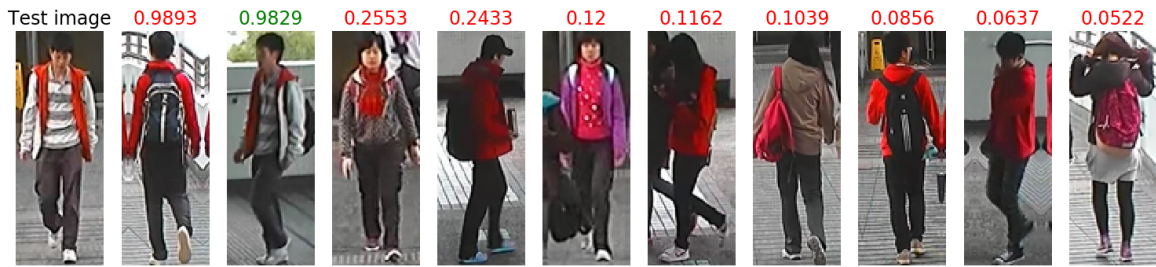
Figure 4.3: To the far left: a test image depicting a test person. To the right: a collection of the ten most probable re-identification matches. Above each image is a similarity score.
