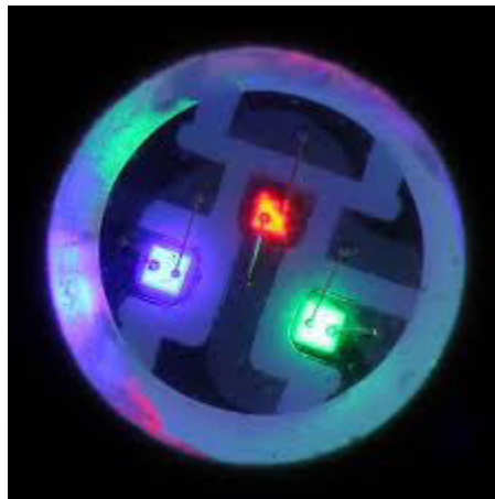
Figure 2. The inside of a diode with three smaller LEDs [3].
