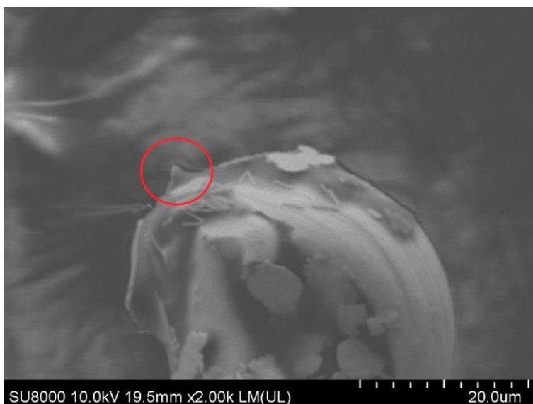
Figure 18. Tip with silver epoxy and clear silver flakes present on the tip. The red circle shows a silver flake extending from the surface.
