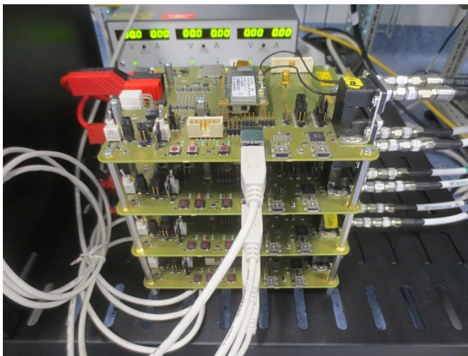
Figure 5.2: UE rack used when testing DL & UL data.
