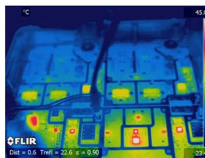
Figure 6.12: Micro Sleep TX enabled. Heat dissipation from the PA are clearly lower.
