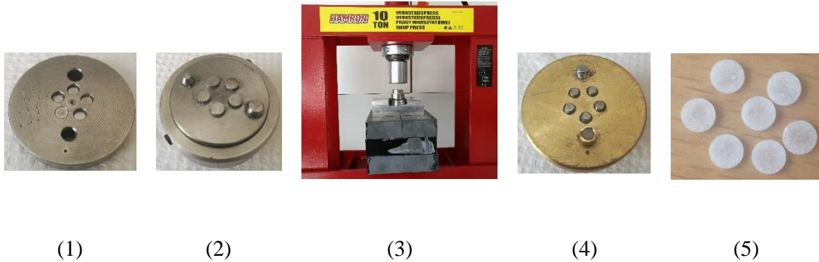
Figure 4. The different parts of the tool which is used to make the NaCl pellets. The salt is placed in the middle cavities of part 1, part 2 is put on top of it and the unit is put under a hydraulic press. Part 4 is used to remove the pellets from part 1. Image 5 shows the final pellets.
