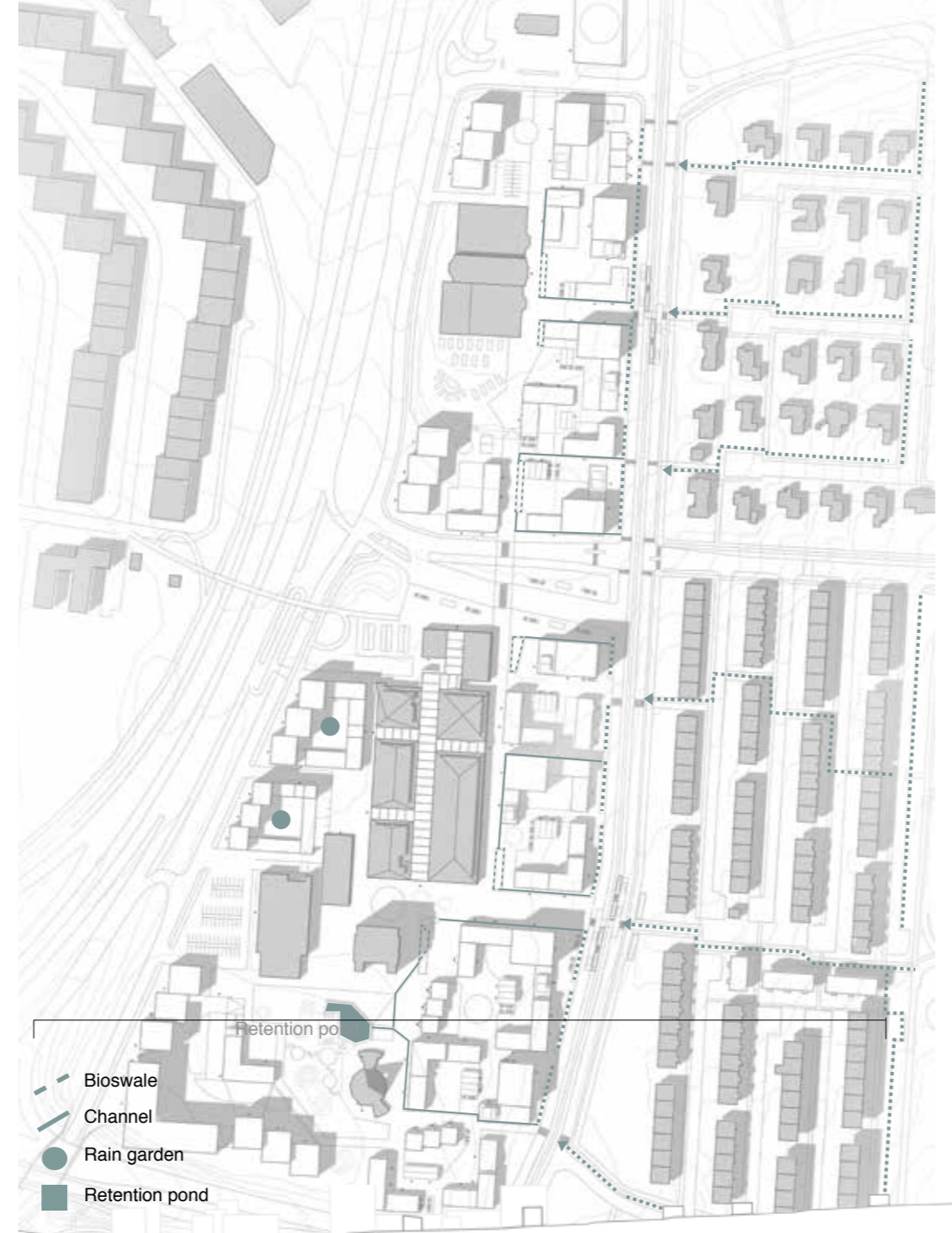
157. Storm water management.
