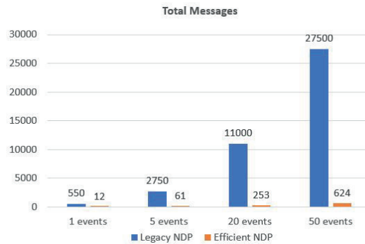
Figure 7.7: Exchanged messages, 50 initial hosts, 10 probes in NUD
