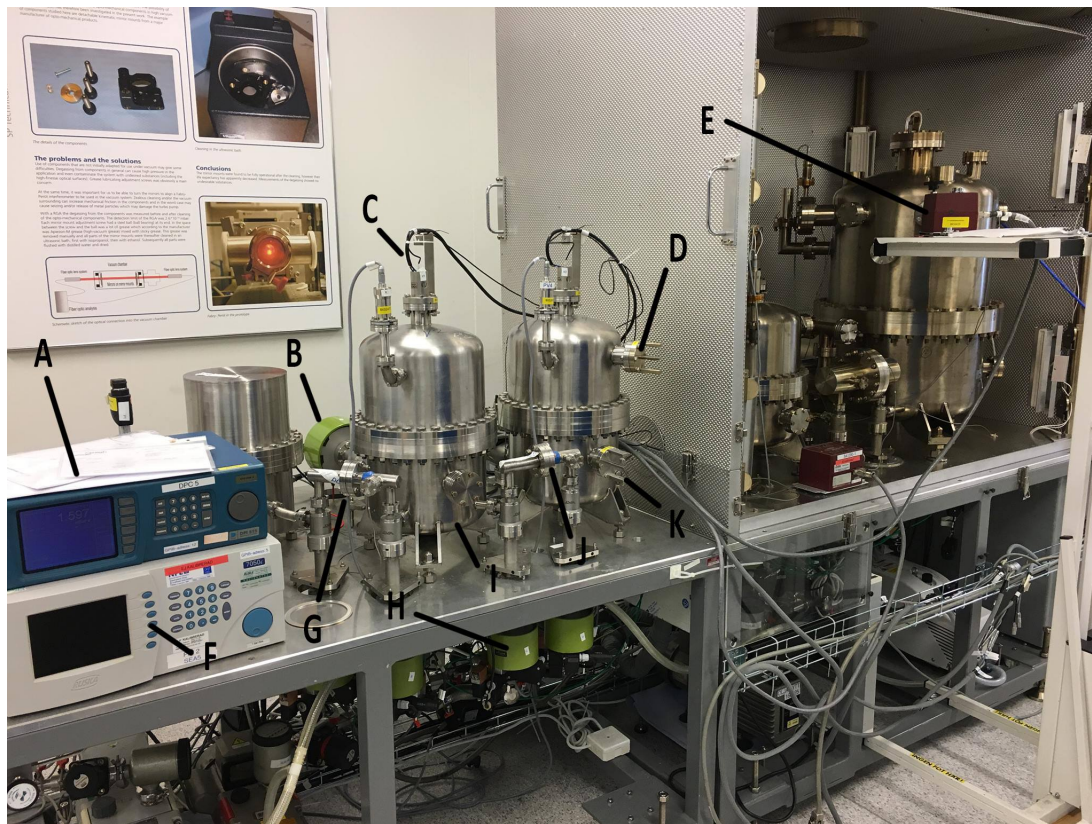
Figure 4.1: A: DPI1515, B: Turbo pump, C: Ionization gauge, D: Connection flange, E: Baratron gauge, F: Ruska 7050i, G: Volume V1, H: Valve, I: Volume V2, J: Volume V3 and K: Volume V4
