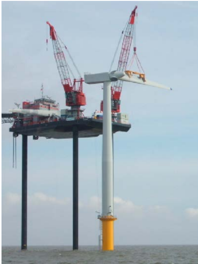
Figure 10. The liftboat Titan 2 (Assessment of vessel requirements for the U.S. offshore wind sector, 2013)
