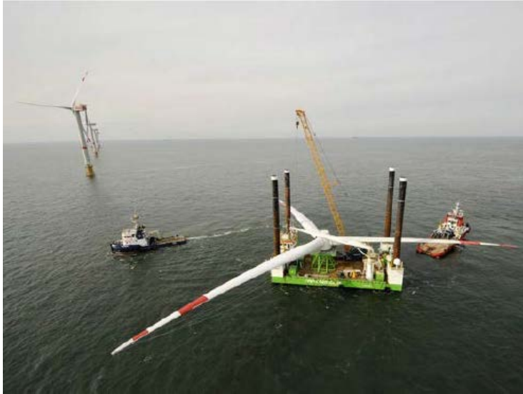
Figure 11. The jack-up barge Vagant is one of the smaller vessels in that class (Assessment of vessel requirements for the U.S. offshore wind sector, 2013)
